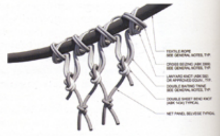
2 TEXTILE ROPE NET CONNECTION DETAIL SCALE: 1/8"
