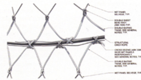
1 STRUCTURAL NET CINCH ROPE CONNECTION DETAIL SCALE: 1/8"
