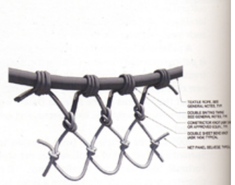
4 TEXTILE ROPE NET CONNECTION ALTERNATE DETAIL SCALE: 1/8"
