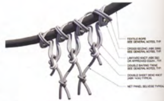
2 TEXTILE ROPE NET CONNECTION DETAIL SCALE: 1/8"
